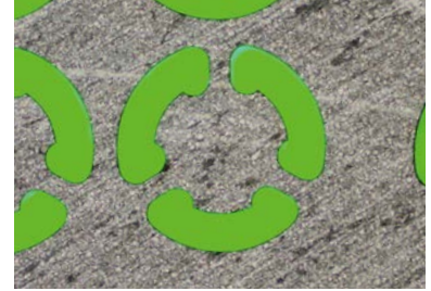
異形孔L長=0.3mm(アスペクト比10倍) ※3種ともに Irregular hole L length: 0.3 mm (aspect ratio 10 times) *For all three types
