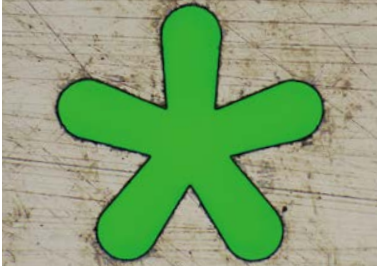
異形孔L長=0.3mm(アスペクト比10倍) ※3種ともに Irregular hole L length: 0.3 mm (aspect ratio 10 times) *For all three types
